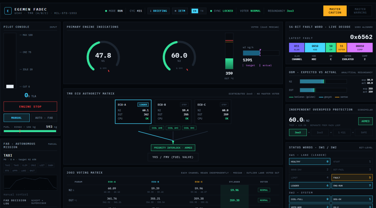
Fig. 2 - Manual idle: N2 held at 60%, all channels healthy, voting NORMAL, OBM residuals hugging zero, fuel full at 600 kg.
